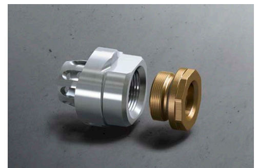
The press-in branch connector is suitable for steel pipes in accordance with DIN EN 10255, DIN EN 10220/10216-1 or DIN EN 10220/10217-1 and available for steel pipe sizes 1½, 2, 2½, 3, 4, 5, and 6 inches. It is provided with an Rp ¾-inch internal thread. A reducer to an Rp ½-inch internal thread is additionally available.
