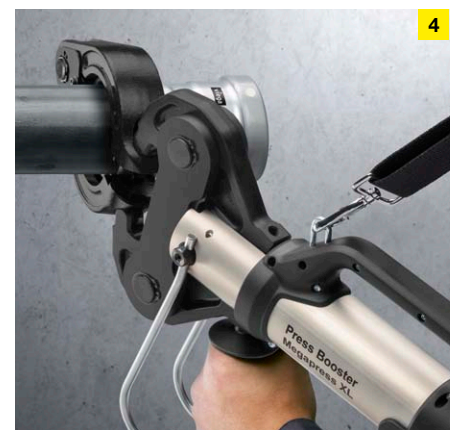
Megapress XL connectors are pressed easily, quickly and safely using a press machine and the Pressgun Press Booster.
