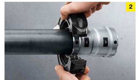
For pressing Megapress connectors from 1\frac{1}{4} inch upwards, only press rings with hinged adapter jaws are used. For smaller sizes between \frac{3}{8} and 1 inch, both press jaws and press rings with hinged adapter jaws are available.
