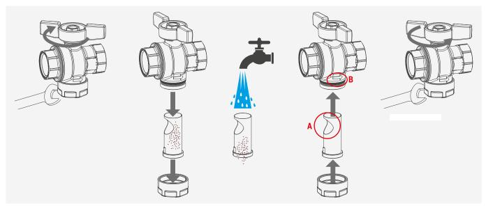
**A** WARNING. After filling the system, we recommend cleaning the filter for the first time after a week of use to remove any obstruction caused by installation residues (metallic chips, seal elements.)
