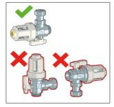
The dirt separator should always be installed horizontally.
