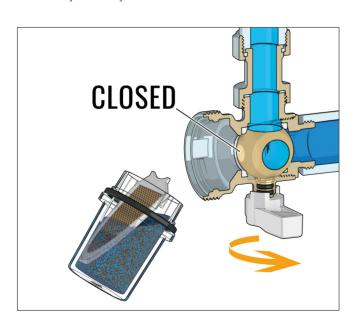
The shut-off valve has been specially designed so that only the water contained in the dirt separator needs to be drained before cleaning the internal elements.
