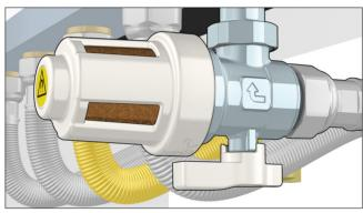
The chamber has transparent windows, so it is easy to check if the internal elements need to be cleaned at any time, and clean them only when strictly necessary.
