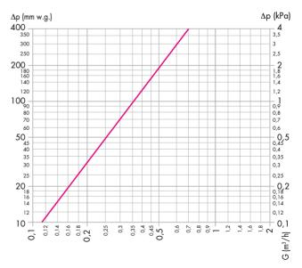
Kv (with clean filter): 3,55 m<sup>3</sup>/h Maximum recommended flow rate: 800 l/h
